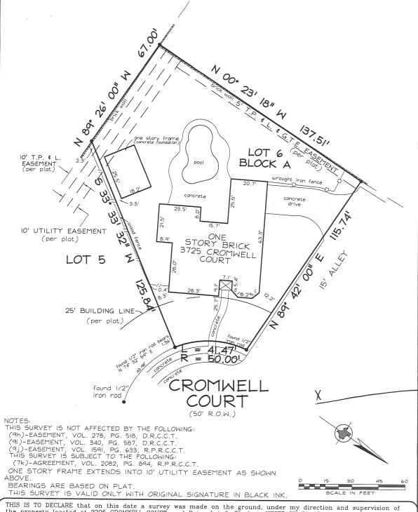
THIS IS TO DECLARE that on this date a survey was made on the ground, under my direction and supervision of the property located at 3725 CROMWELL COURT, and Being Lot 6, Block A, WESTPARK PLACE NO. 6, an Addition to the City of Plano, Collin County, Texas, according to map or plat thereof recorded in Volume F, Page 250, of the Plat Records of Collin County, Texas.
