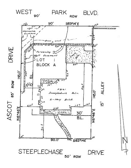
The plat hereon is a true, correct and eccurate representation of the property as determined by survey, the line; and dimensions of said property being as indicated by said plat, the size, incution and type of buildings and improvements are as shown, all improvements being within the boundaries of the set back from property lines the distance indicated and that the distance to the normal street or road is as shown.
